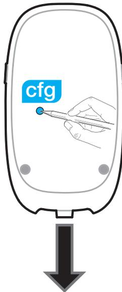
**i** All time switches (output) enter configuration mode.
