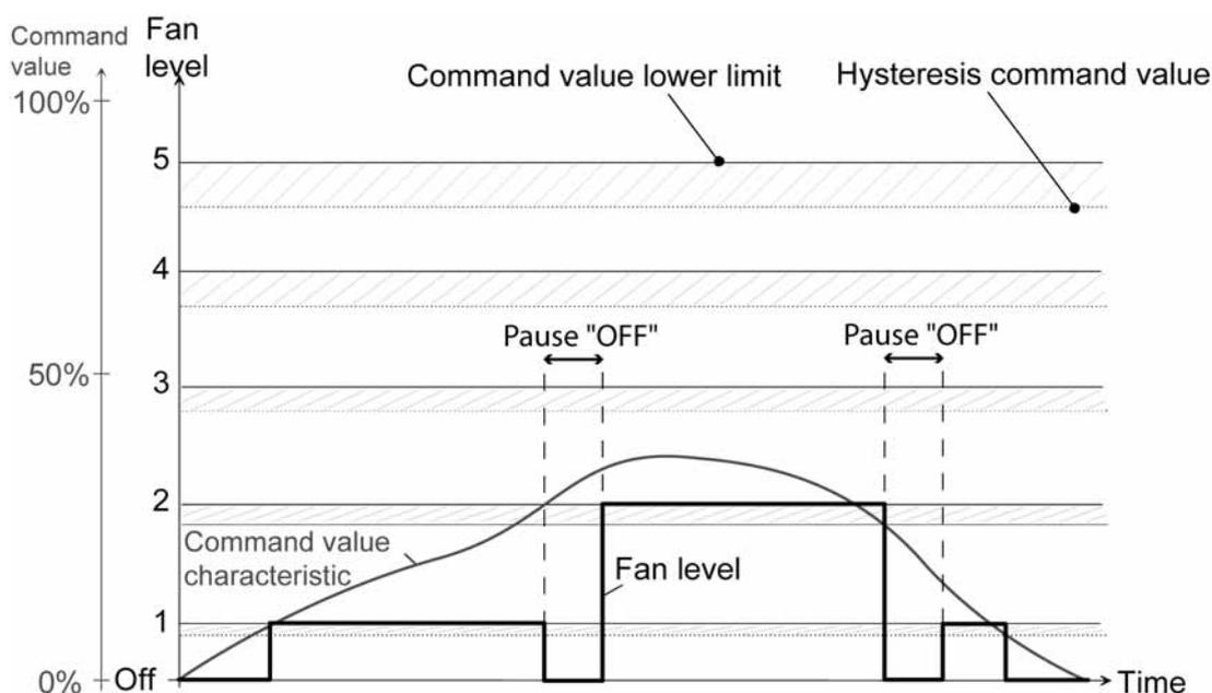
picture 25 Simplified command value diagram to illustrate a fan level change-over with the change-over principle, taking into account the pause "OFF" 1
