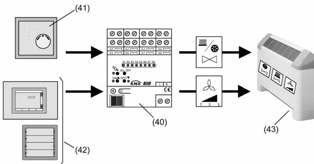
picture 28 Principle of manual fan control
