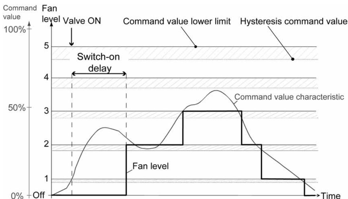
picture 23 Simplified command value diagram to illustrate a fan level change-over (active fan level), taking into account a switch-on delay
