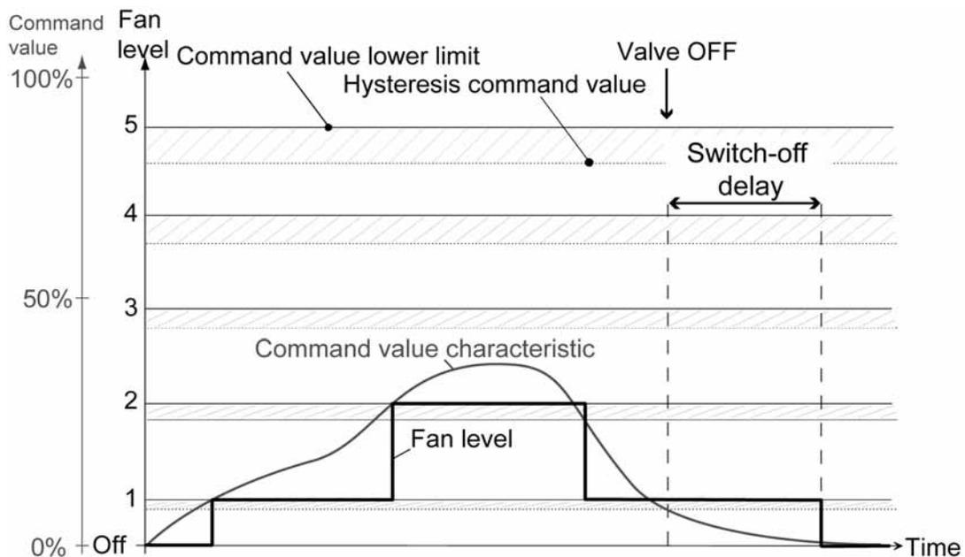
picture 24 Simplified command value diagram to illustrate a fan level change-over (active fan level), taking into account a switch-off delay
