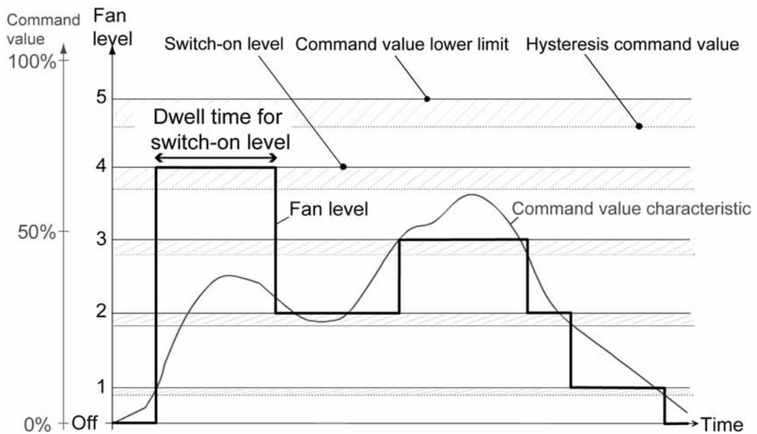
picture 22 Simplified command value diagram to illustrate a fan level change-over (active fan eve ), taking into account the switch-on level
