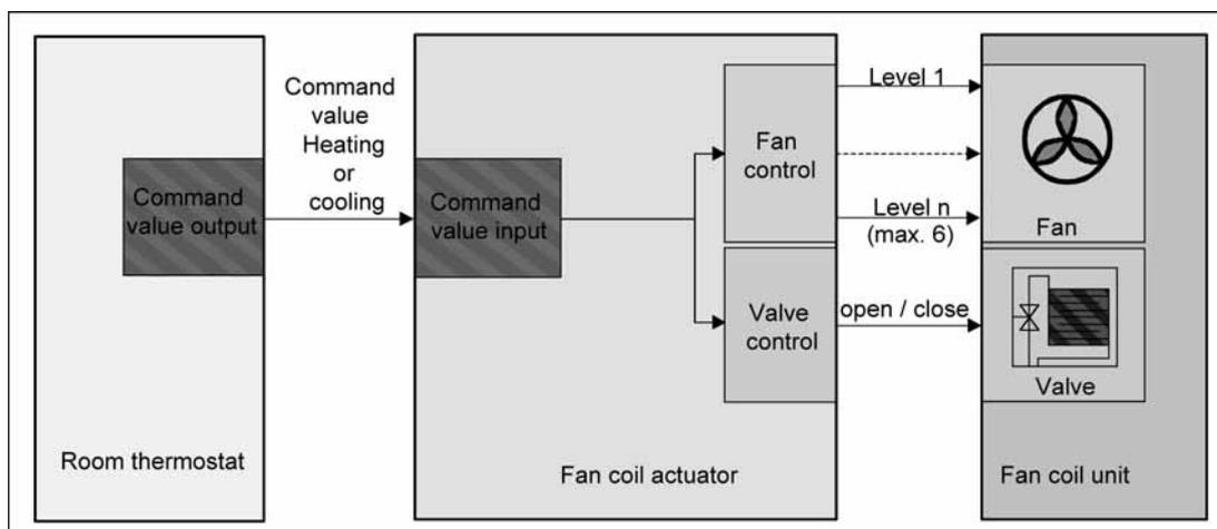
picture 12 Functional diagram for "2-pipe on y heating" and "2-pipe only cooling"
