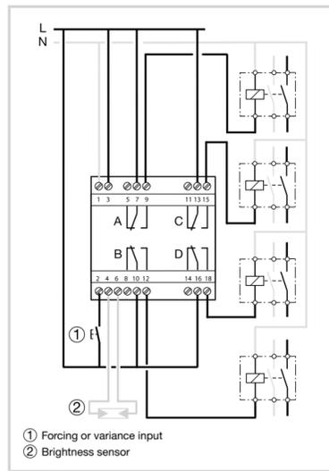
Image 3: EGN400 connection diagram (4 outputs)
