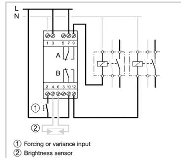
Image 2: EGN200 connection diagram (2 outputs)
